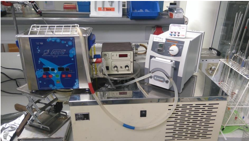
Figure 3-4 Ultrasonic extraction system (source: private collection)
