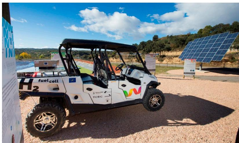
**Figure 9.** The fuel cell hybrid electric vehicle (FCHEV).
