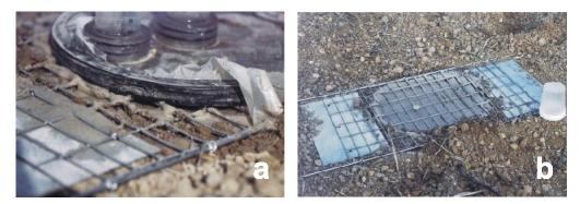
Figure 3.4. Soil collapse during (a) and at the end (b) of infiltration at saturation with disc infiltrometer *Mode 3* on a structureless soil.
