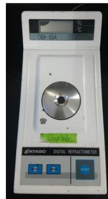
**Figura 8:** Digital Refractometer DBX-55A, Atago.
