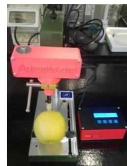
**Figura 7:** Digital Penetrometer Agrosta@14 Field.
